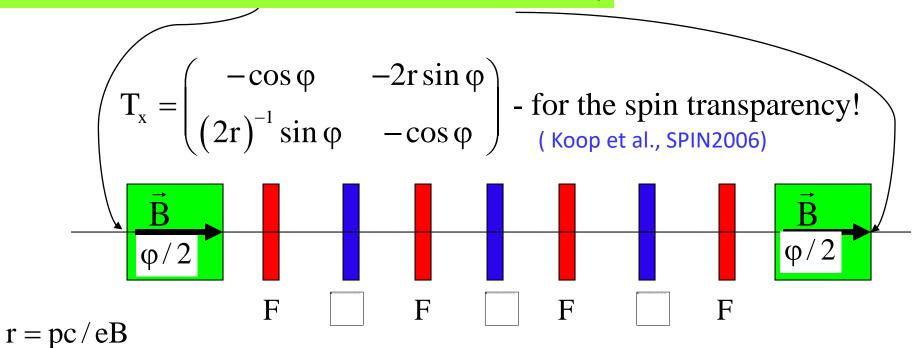
Two solenoids rotate spin by the angle φ
