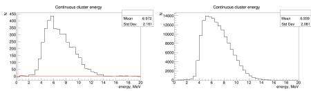
The continuous cluster energy: measured data (left), simulated decays of boron (right)
